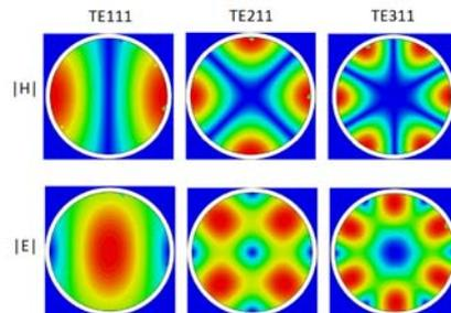
Fig. 1 – Magnetic (H) and electric (E) field distribution for several modes in the cross section of a cylindrical waveguide resonator.
