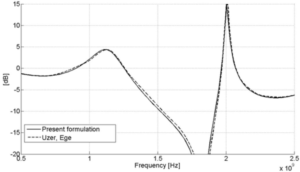
**FIG. 2** – Ratio (dB) between radiated power measured away from the electric line current, with and without the CFSS, with  $N = 16$  circumferential patches and unit cell parameters:  $b = 50$  mm,  $T_z = 100$  mm,  $l = 90$  mm,  $w = 4$  mm.
