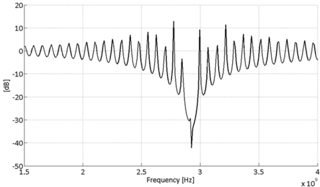
**FIG. 3** – Same as in Fig. 2, for  $N = 250$  circumferential patches, and unit cell parameters:  $b = 50$  mm,  $T_z = 55$  mm,  $l = 50$  mm,  $w = 4$  mm.
