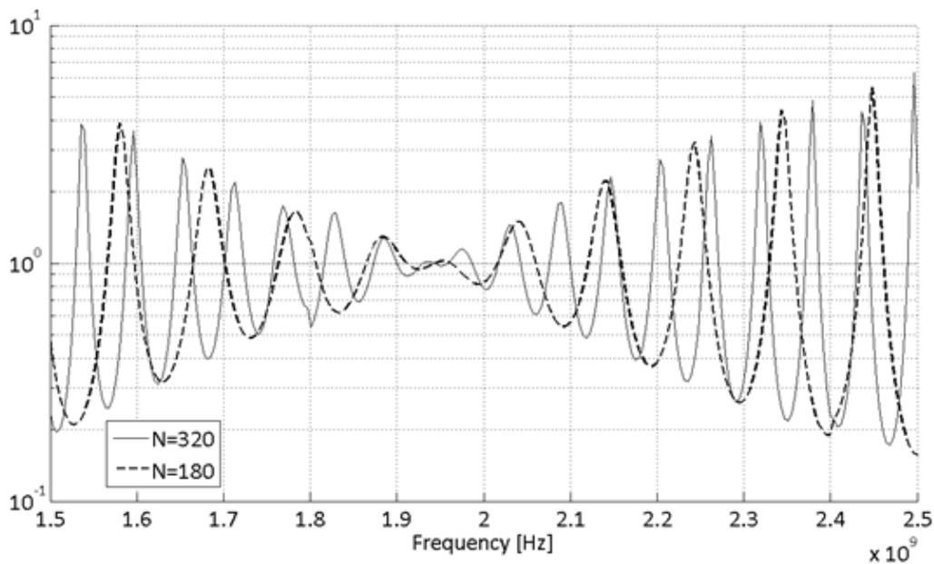
**FIG. 4** – Ratio between longitudinal magnetic field (magnitude) measured away from the magnetic line current, with and without the CFSS, presenting 180 or 320 circumferential slots and:  $b = 50$  mm,  $T_z = 100$  mm,  $l = 90$  mm,  $w = 4$  mm.
