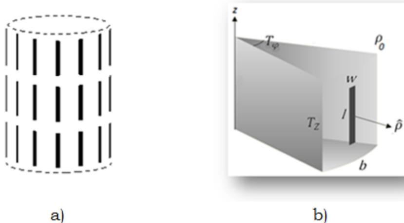
**FIG. 1** – a) Cylindrical Frequency Selective Surface, made by conducting patches or slots; b) relevant unit cell parameters.
