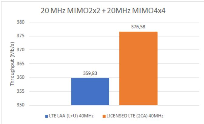
Fig. 4. Comparison LTE vs. LTE LAA in 40 MHz
