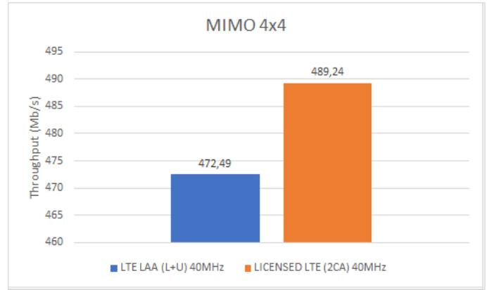
Fig. 5. Comparison LTE vs. LTE LAA in MIMO 4x4
