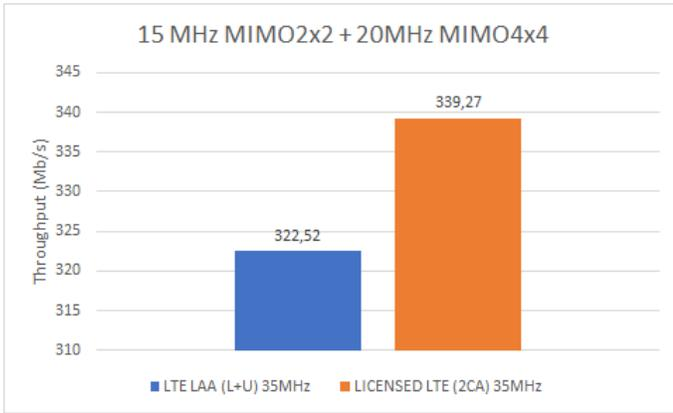
Fig. 3. Comparison LTE vs. LTE LAA in 35 MHz
